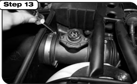
Step 13 Tighten clamp on tube and align bolt holes on tube to housing.
