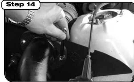
Step 14 Use the three M6 x 1 x 25 screws, flat & wavy washers provided to bolt the tube flange to the housing.
