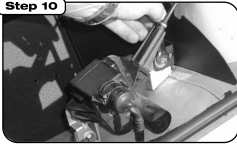
Step 10 Place cruise control module back in location and use M6 x 1 x 16 screws, washers supplied with kit.
